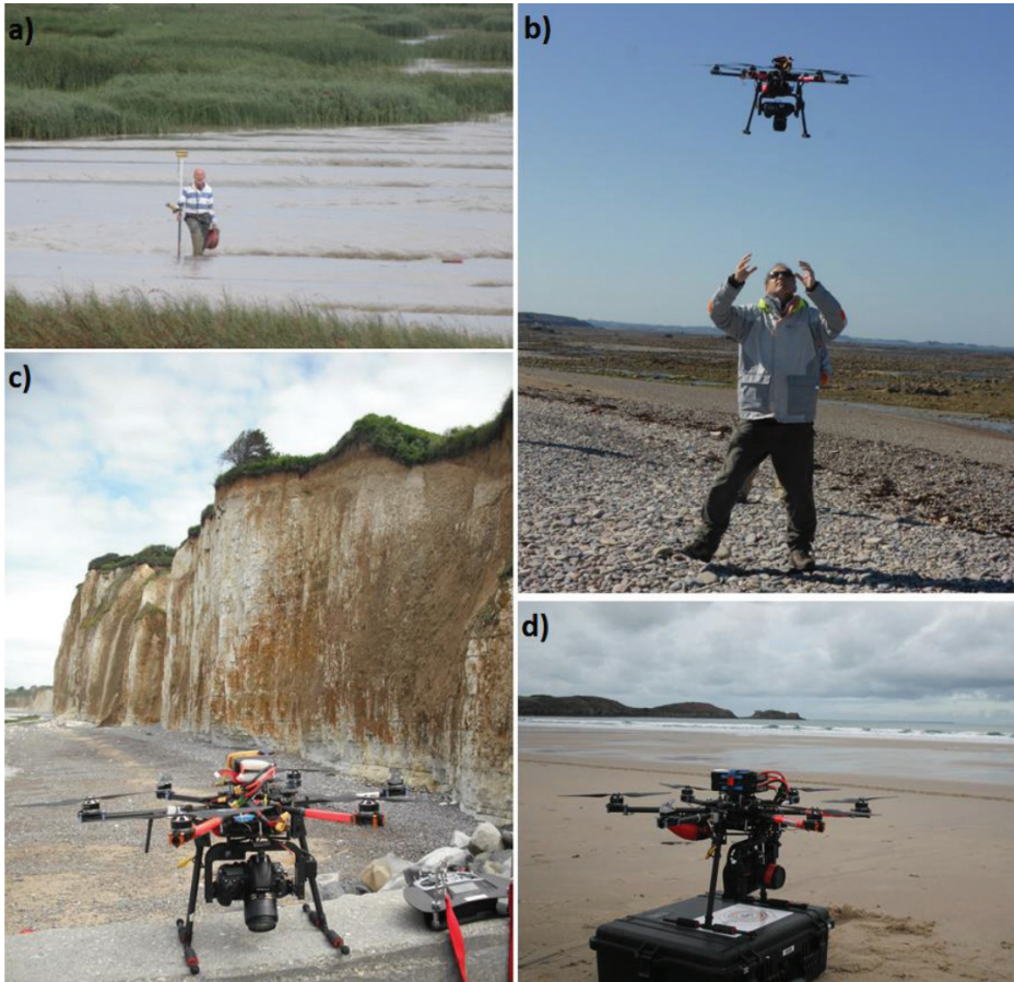
Figure 6: Performing UAV surveys in different coastal environments: (a) estuarine mudflat, (b) pebble beach, (c) cliff, (d) sandy beach
