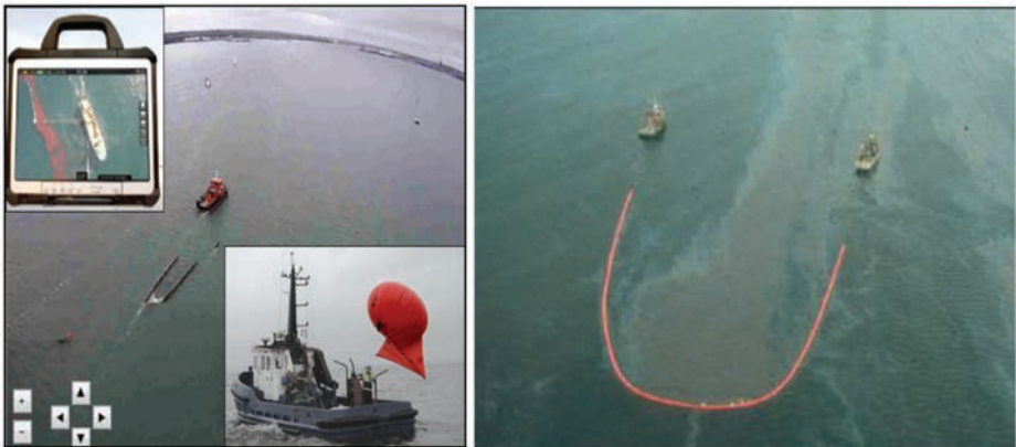
Figure 5: Offshore survey using tethered balloons
