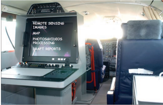
Figure 4: Computer inside the F406 POLMAR III
