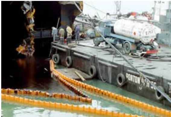
Booms used for confinement and recovery by empty tanks ©CEDRE
