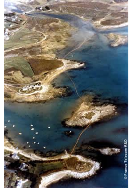
Aerial view of booms setup to protect the coastline ©France Telecom R&D
