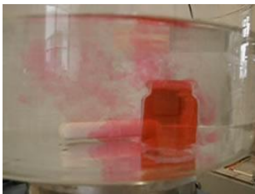
2. Slow dissolution of the acid after opening the jar, without agitation ©CEDRE
