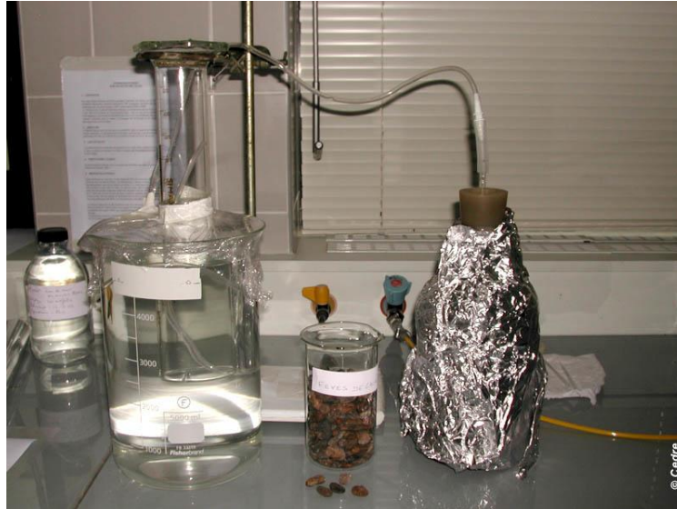
Experimental device for the collection of gas emissions ©CEDRE
