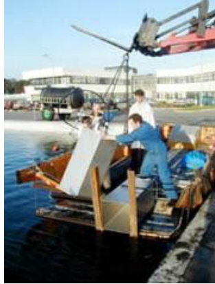
Immersion of stainless steel tanks in an outdoor sea water basin ©CEDRE
