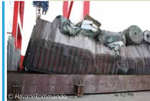
Container and cargo damaged by the fire/heat
