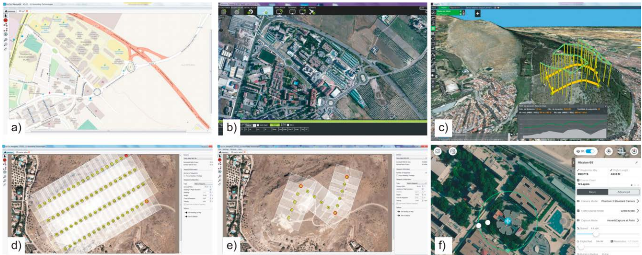
Figure 2-7. Examples of photogrammetric mission planning software: (a) Astec Navigator using OpenStreetMap; (b) Mission Planner displaying Bing Aerial Image; (c) UgCS planning module using a block flight determined by a polygon limit using a DEM; (d) image footprints in Astec Navigator block flight; (e) image footprints in Astec Navigator corridor flight; and (f) circular flight planning in DJI GS Pro. (From Gómez López et al., 2020).
