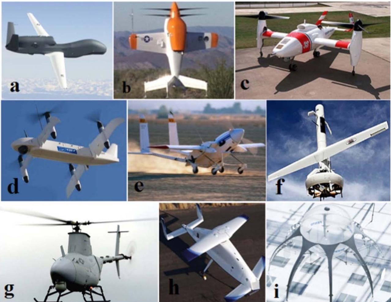
Figure 2-4 Different types of UAVs, (a) HTOL, (b) VTOL, (c) tilt-rotor UAV, (d) tilt-wing UAV, (e) tilt-body UAV, (f) ducted fan UAV, (g) helicopter, (h) heli-wing, and (i) unconventional UAV (source: Hassanalian and Abdelkefi, 2017).
