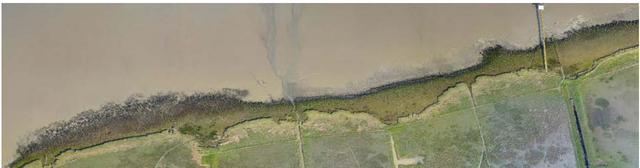
Figure 5-3. Photomosaic (scenario 1, flight altitude 110 m, pictures overlap ratio 70%)
