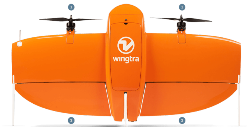
Figure 2-6. An example of fixed-wing VTOL UAV ( https://wingtra.com/ )
