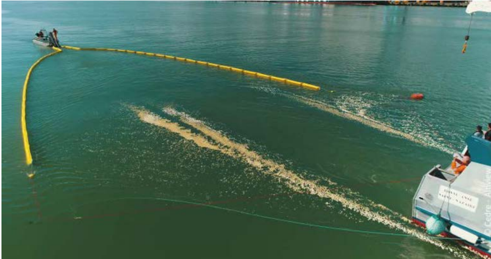
Figure 5-1 and Figure 5-2.. Use of the drone to guide the recovery boat (source AltiView)
