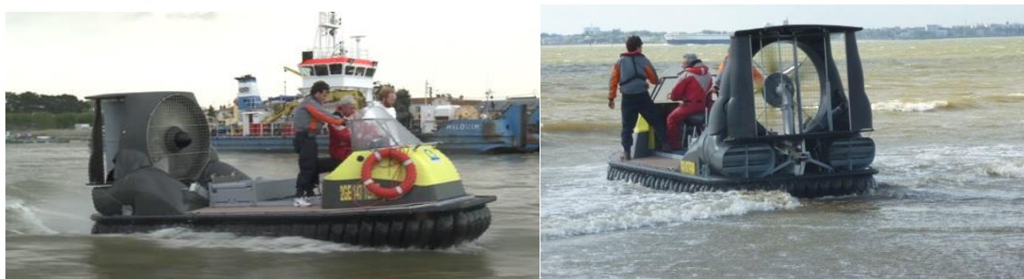
Figure 3. Tests (Loire estuary): platform stability on water at high speed, and at the water edge.
