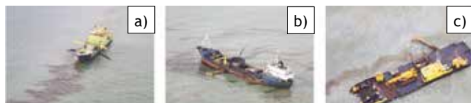
Figure 11: Oil spill response at sea during the Flinterstar : (a.) ARCA; (b.) INTERBALLAST I; (c.) HEBOCAT 7.
