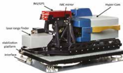
Figure 4: Airborne platform for flying the Hyper-Cam instrument in a fixed-wing aircraft [4]
