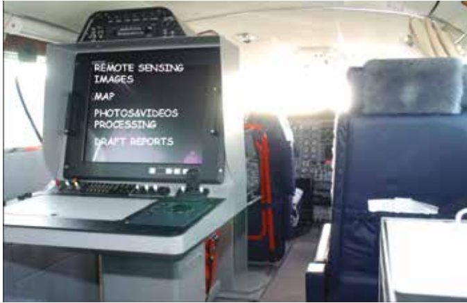
Figure 4: Computer inside the F406 POLMAR III
