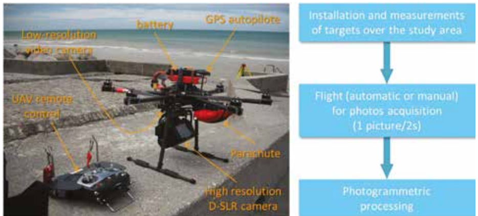
Figure 3: DRELIO 10 system configuration and main steps during a drone survey.
