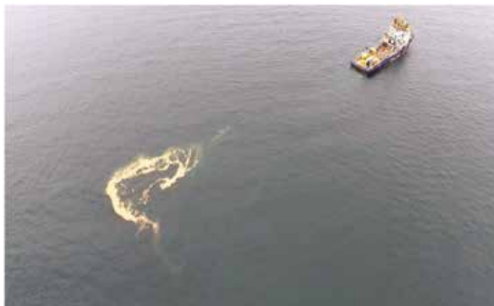
Figure 2: Visual detection of rice husk from 100m altitude (SUAS: 3DR Solo & Gopro 3+Black)
