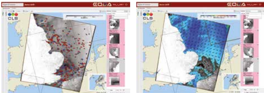
Figure 2: (Left) Vessel detection reports with two classes of confidence and (Right) SAR derived wind fields
