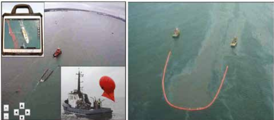
Figure 5: Offshore survey using tethered balloons
