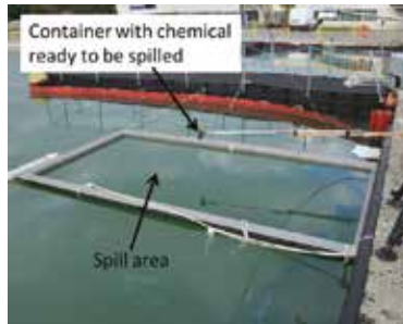
Figure 3: Region of the spill area viewed by the Hyper-Cam, and the container with the chemical to be spilled into the seawater by Cedre personnel
