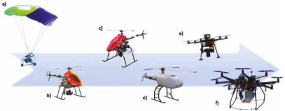
Figure 2: Various models of drones implemented by the laboratory Domaines Océaniques since 2006: (a) Pixy wing, (b), (c), (d) thermal helicopters, (e) hexacopter, (f) octocopter.
