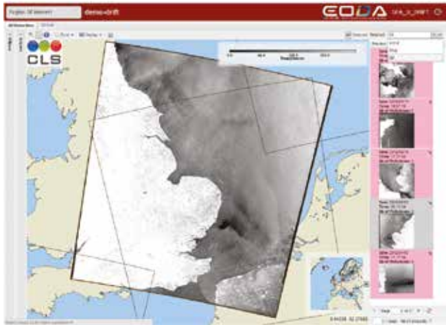
Figure 3: Sea surface roughness and oil spill
