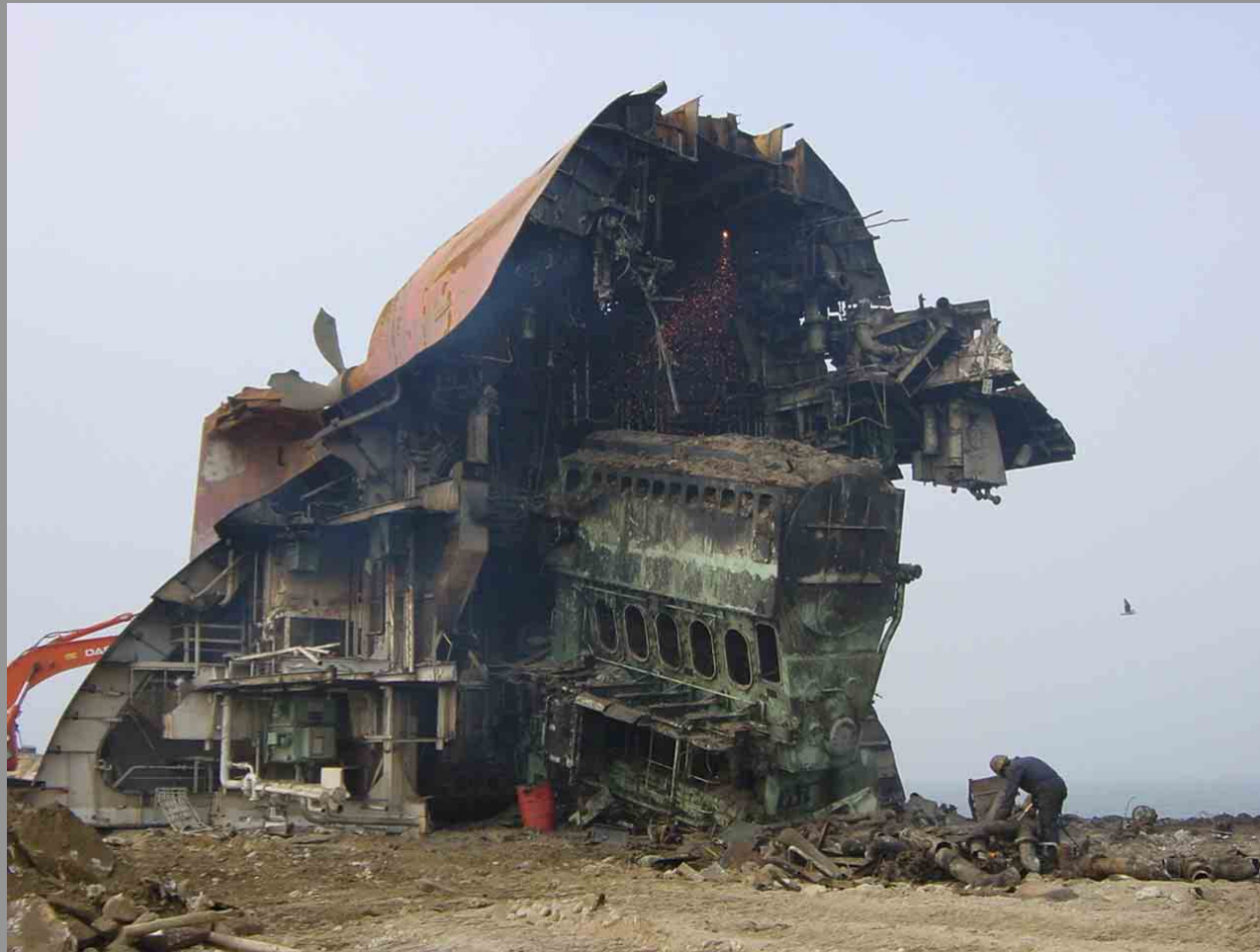
SCRAPPING REMAINS OF STERN SECTION AT BREAKWATER SITE
