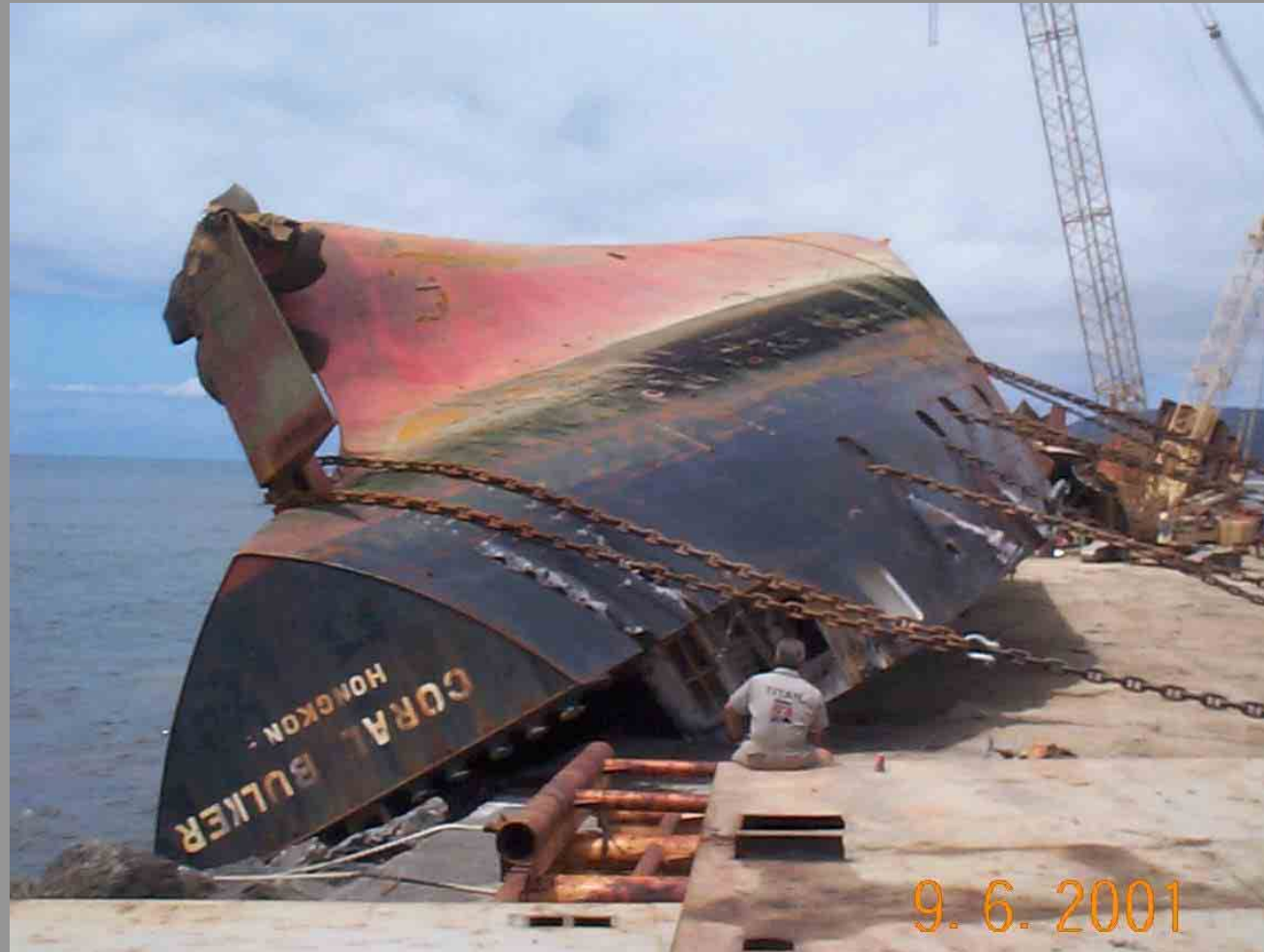
STERN SECTION ROLLED ONTO BREAKWATER
