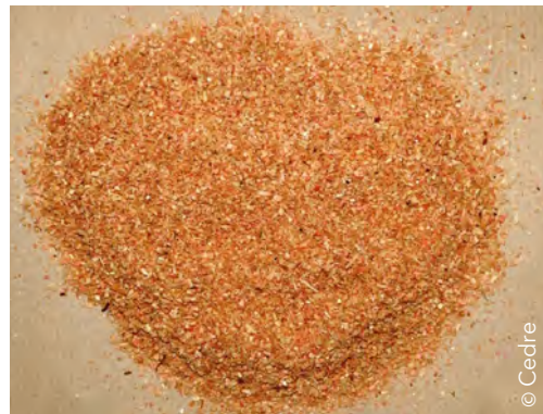
Bulk sorbents are used (in confined areas) to increase the thickness and viscosity of liquid on the sea surface or to intervene on solid polluted surfaces.
