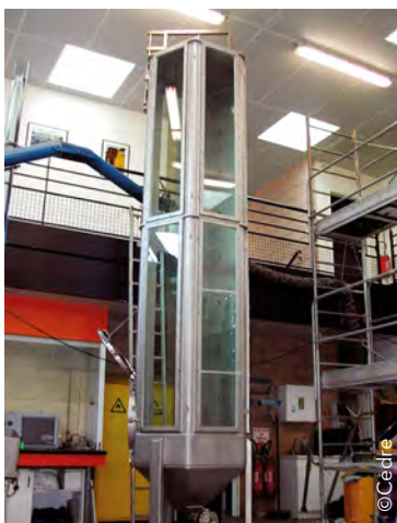
Experimentation column to study the behaviour of a chemical (or oil) as it rises or sinks in the water column.
