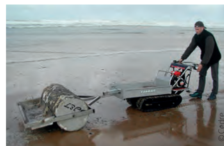
▲ Demonstration of an oleophilic roller pushed by a caterpillar-tracked trolley, Gironde
