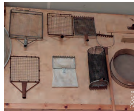
^ Examples of custom-made skimming devices made by Spanish fishermen on display in Cedre's showroom
